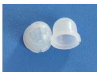
型号:011050 焦距:5mm 尺寸:Φ 11.8*9.9 感应角度:120° 感应距离:5-6m
