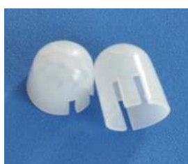
型号:8308-2 焦距:6mm 尺寸:Φ 11.5*14.5 感应角度:60° 感应距离:5m
