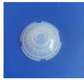
型号:8605-12 尺寸:Ø43.8 焦距:17mm 感应角度:360° 感应距离:直径 10m
