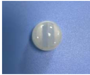
型号:8121-5 尺寸:Φ9.8 感应角度:120° 焦距:5.2mm 感应距离:8m
