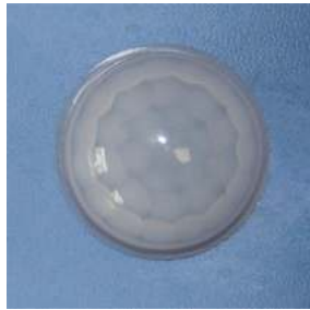
型号:8003-2F-X 尺寸:25.5*12.3 焦距:10.5mm 感应角度:120°感应距离:10m
