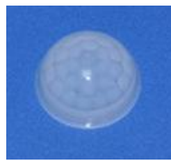
型号:8003-2F 焦距:10.5mm 尺寸:Ø 25.3*12.5 感应角度:120° 感应距离:12m
