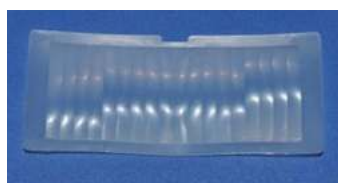
型号:7707-1A 尺寸:91.3*39.5 感应角度:180° 焦距:25mm 感应距离:16m
