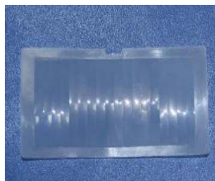
型号:7707 感应角度:180° 焦距:25mm 感应距离:16m 尺寸:91.3*39.5
