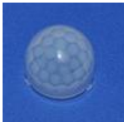
型号:8005-2感应距离:10m 尺寸:Φ 23*19.7 焦距:11mm 感应角度:120°
