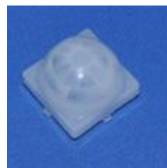
型号:023100 感应距离:10m 尺寸:23.4*23.4*18.9 焦距:10.5mm 感应角度:120°
