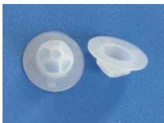
型号:008140 焦距:5.5mm 感应角度:90° 感应距离:4m 尺寸:Φ 13.2*5.5
