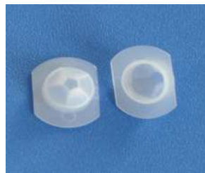
型号:008140-G 焦距:5.5mm 感应角度:90° 感应距离:4m 尺寸:13.2*10*5.5
