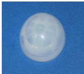
型号:023101 焦距:10.5mm 尺寸:Ø 23.4*11.5 感应角度:120° 感应距离:10m
