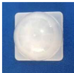
型号:023100去腿焦距:10.5mm 尺寸:23.4*23.4*18.9 感应角度:120°感应距离:10m
