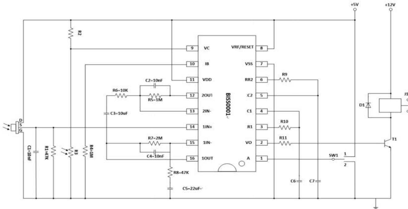
**8脚处理芯片典型应用电路 Typical application circuit of 8-pin processing chip**
